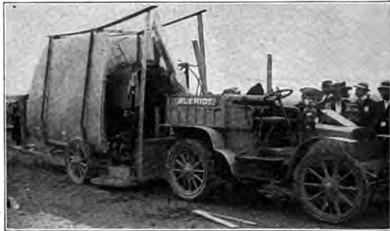
Fig. 2. Bleriot Military Monoplane, Showing Portability Feature
